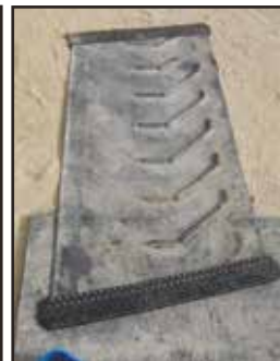
Bridge repair old belt with new belt
