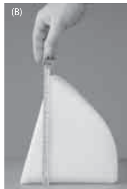
With elevator bucket back laid flat, measure the horizontal projection of the elevator bucket (B).
